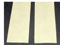
25 mm strips of OPPANOL® adhesive films for FINAT tests
