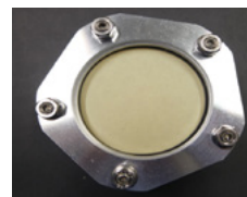
Water Vapor Transmission Test
